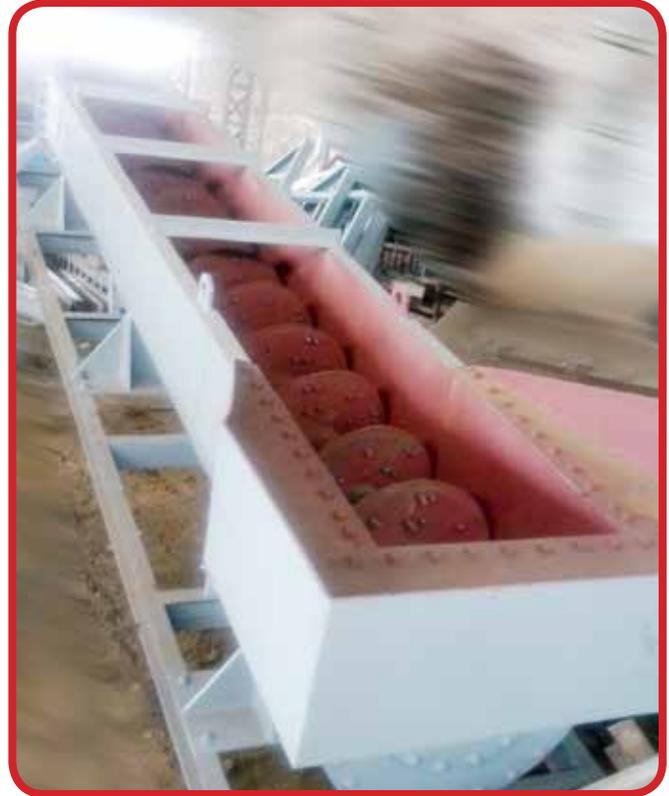
solids to settle out, whereupon they are removed by mechanical means. Solids that do not settle report as overflow from the pool. Up gradation of 2 to 3% is achieved improving qualities of end product. We offer wide range of spiral classifier, industrial spiral classifier, industrial spiral separator, solid liquid separators and spiral separator.
